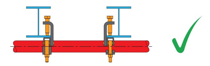
Girder couplers must not be clamped on the same side of the structural sections.
